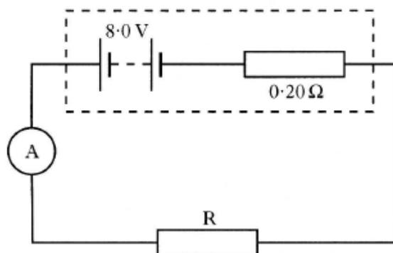
The reading on the ammeter is  $4.0\text{ A}$ .
