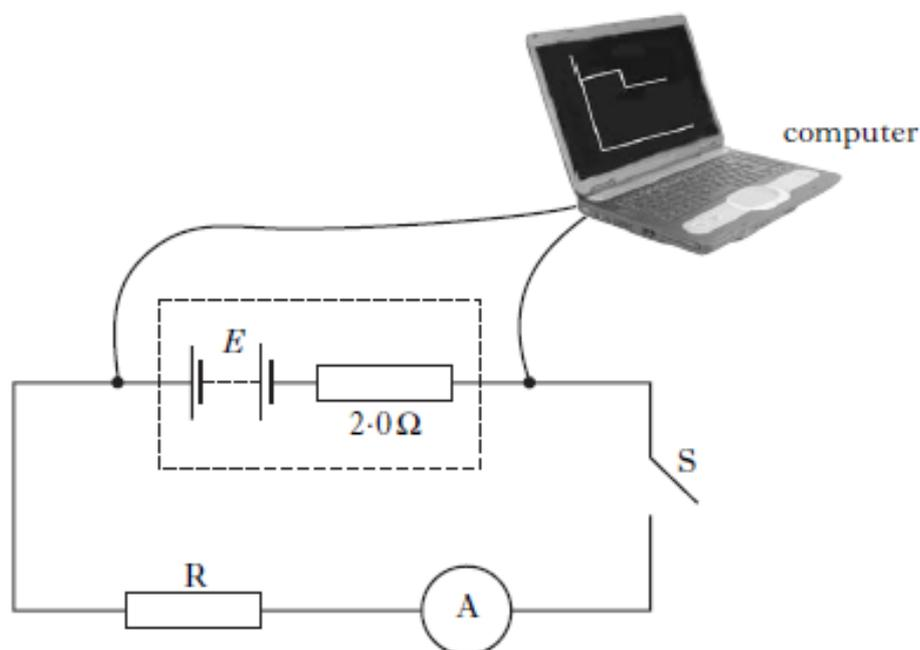
The computer connected to the apparatus displays a graph of potential difference against time.
