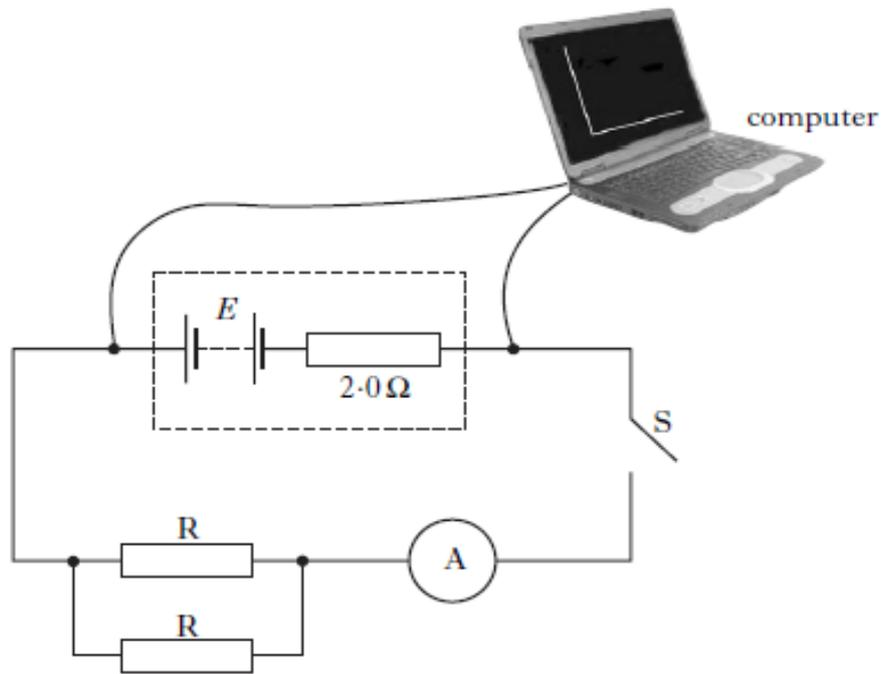
The computer is again connected in order to display a graph of potential difference against time.
